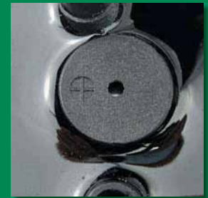
Externally controlled built-in piezo sounder
