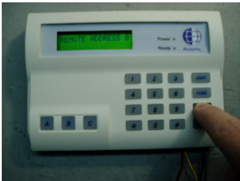
To display the current remote address press and hold the BAT button for about 3 seconds.
