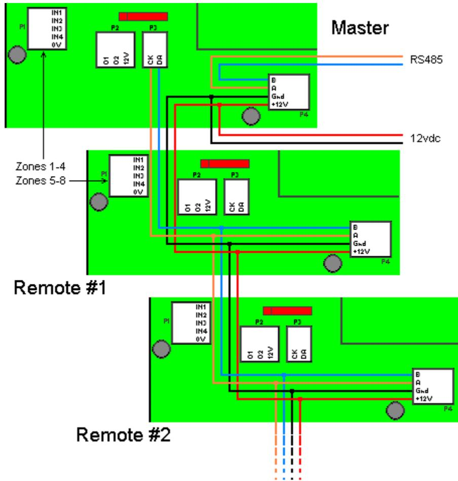
Add wires to the CK and DA terminals on the master and connect in parallel along with power to the slaves.
