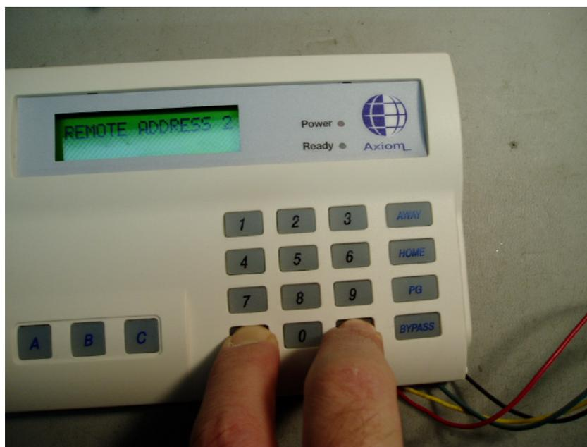
To change the address, hold the \* and # buttons down for about 3 seconds.
